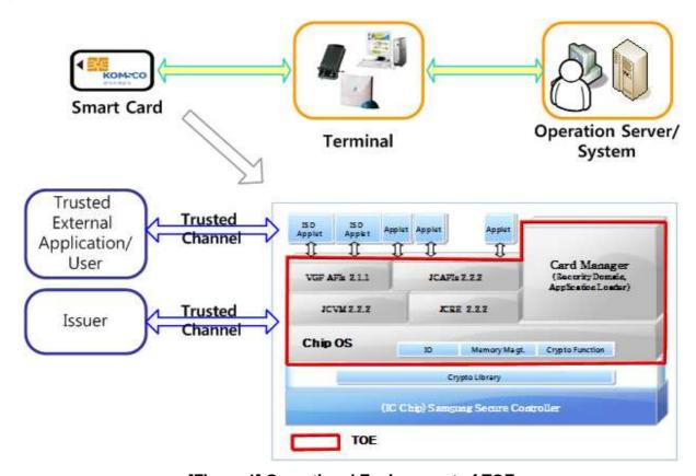
[Figure 1] Operational Environment of TOE
