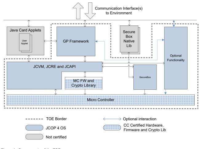
Figure 1. Components of the TOE
