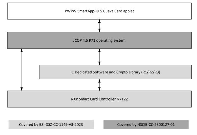
The TOE is a composite product comprising the application implementing the security functionality of the TOE by relying of the underlying certified OS functionalities coming from the JCOP OS running on the HW IC. For each of the security functionalities, the application implements a subsystem with the according functionality. Those subsystems interact together to ensure the TOE functionality in terms of TOE architecture.
