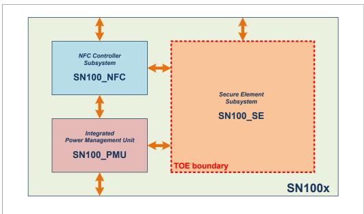
Figure 1. Toplevel block diagram of SN100x
