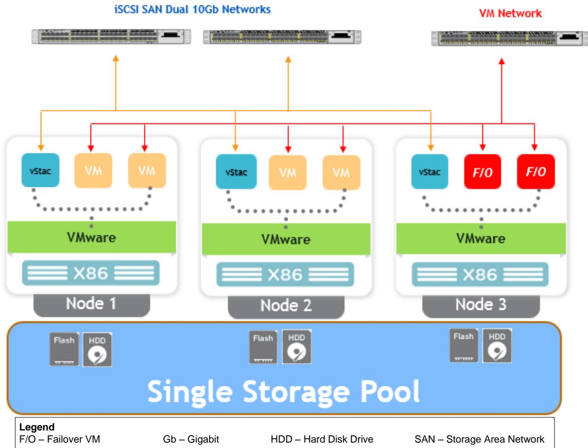
**Figure 1 – Pivot3 Hyperconvergence Architecture**
