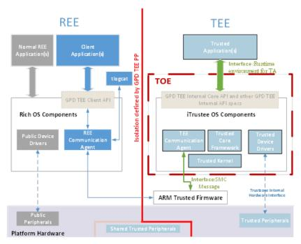
Figure 1 The architecture of a TOE-enabled device
