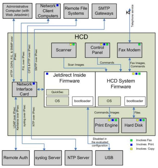
Figure 1: HCD physical diagram
