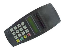
The C-ZAM/DEP is a chip card encoder/reader with its own keyboard and display. It is used for administration purposes and uses smart cards (called DCCs: DEP Control Cards) to store information relevant for securely administering the TOE. The C-ZAM/DEP itself is not part of the TOE and falls outside the scope of the evaluation.
