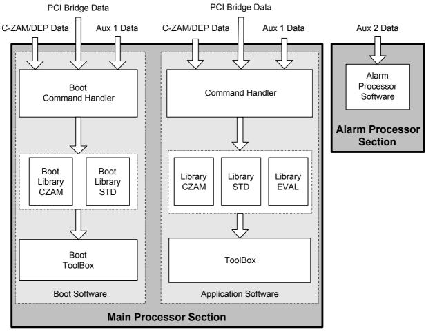
Figure 3: TOE-Software Environment
