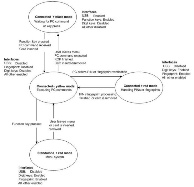
Figure 3: Modes of operation for BioSec Reader
