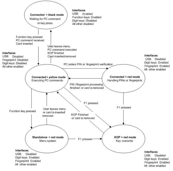
Figure 2: Modes of operation for KT2USB reader
