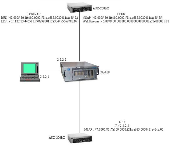
Figure 1 Test Bed Setup 1
