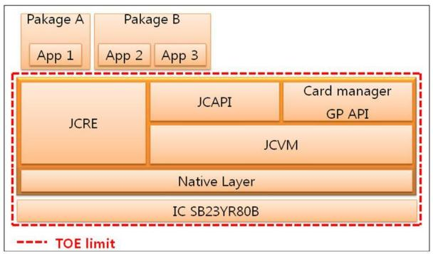
Figure1. TOE Architecture
