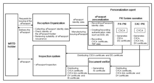
Figure 2 Entire Composition Diagram of ePassport System
