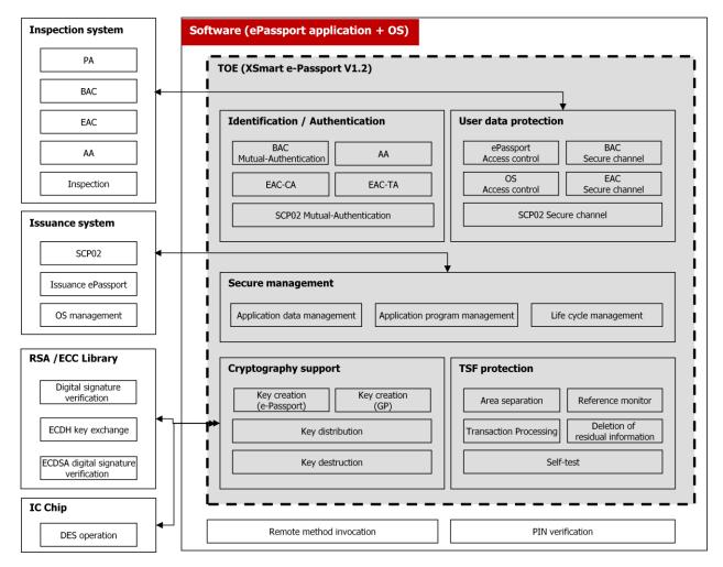
Figure 6 Logical Scope of TOE
