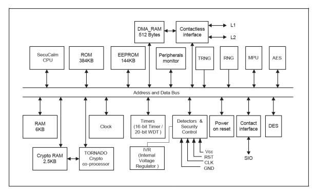
**Figure 3 IC Chip Hardware Composition Diagram**
