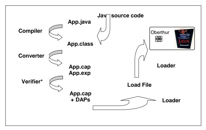
Figure 4: Tools used before delevery applet (compiler, converter, verifier, and loader)
