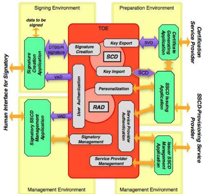
Figure 3: TOE and operational environments with Key Import
