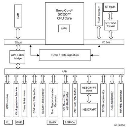
Both hardware support an SPI interface compliant with [11] for integration with controllers and system drivers.
