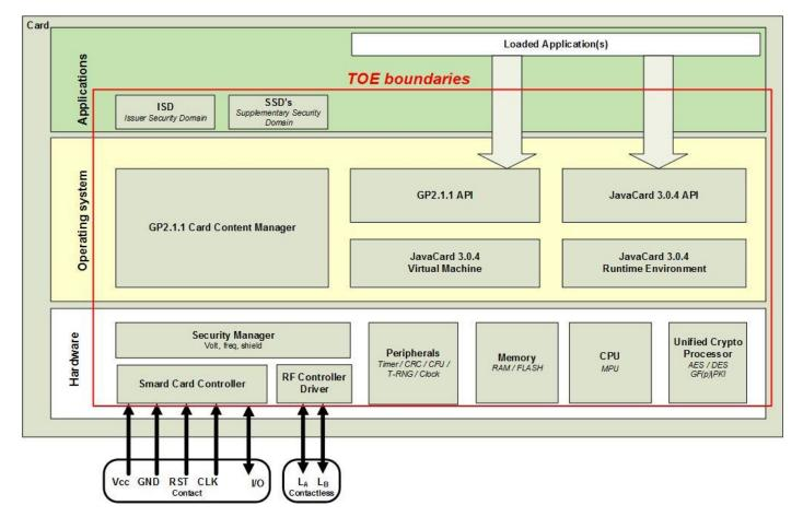
Figure 1 View of the smartcard and pins
