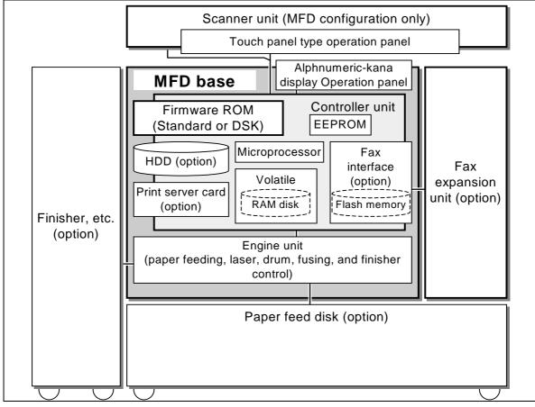
Figure 1: The TOE and physical configuration of the MFD
