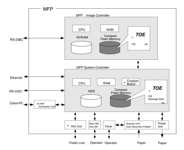
Figure 2 Hardware composition that relates to TOE
