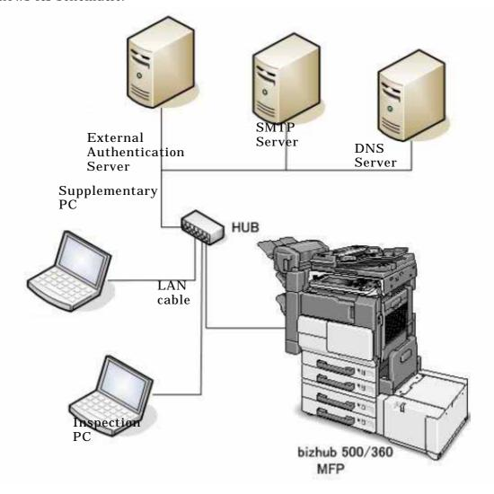
Figure 2-2 Developer test (Intrusion test) configuration
