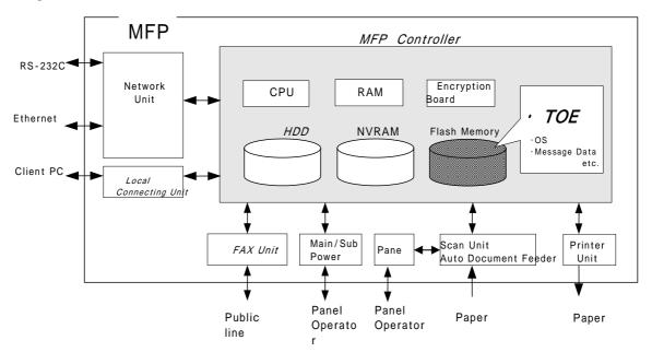
Figure 1-1: Hardware structure that relates to TOE
