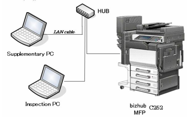
Figure 2 2 Developer test (Intrusion test) configuration
