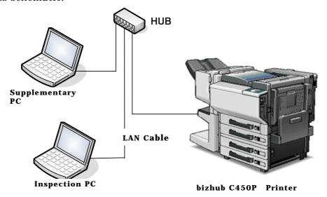
Figure 2-2 Developer test (Intrusion test) configuration
