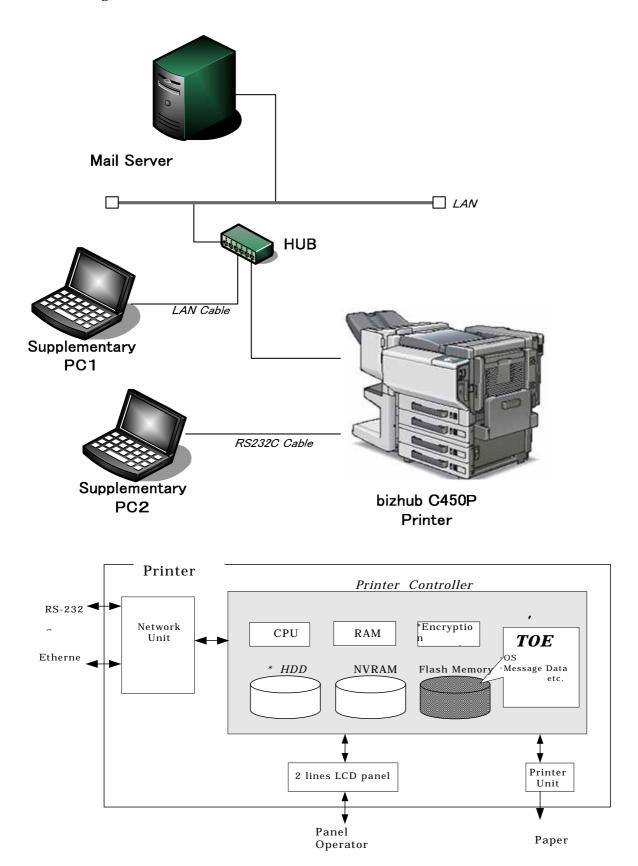
Figure 2-1 Configuration of Developer Testing
