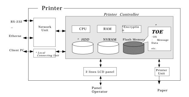
Figure 1-1: Hardware structure that relates to TOE
