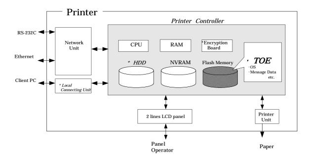
Figure 2 Hardware composition that relates to TOE
