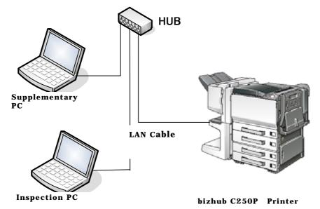
Figure 2-2 Developer test (Intrusion test) configuration
