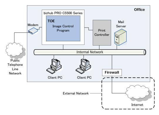
Figure 2-1 Configuration of Developer Testing
