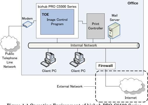
Figure 1-1 Operating Environment of bizhub PRO C5500 Series
