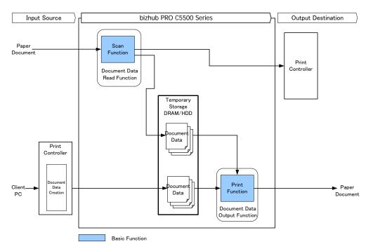
Figure 1-3 Processing Architecture of Basic Function
