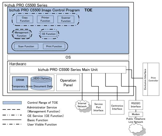
Figure 1-2 TOE Structure
