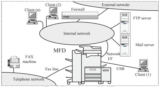
Figure 3: Usage environment of the MFD
