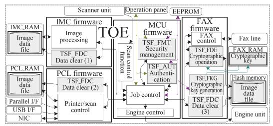
Figure 2: Logical configuration of the TOE
