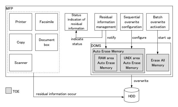
Figure 4: The MFP and the TOE functions and those relations
