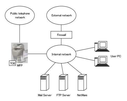
Figure 1: Operational environment of the MFP
