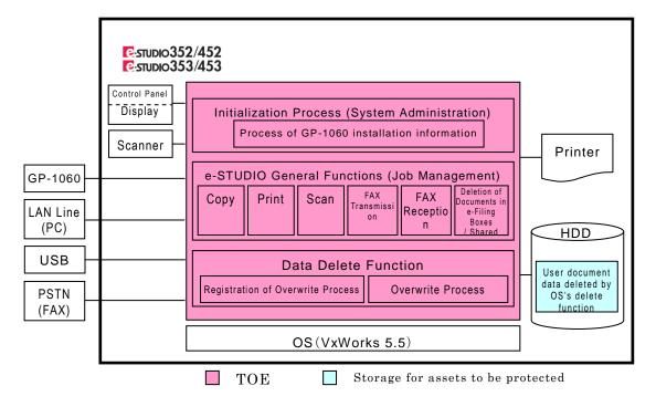
Figure 1-2 Product Configuration in Normal Mode
