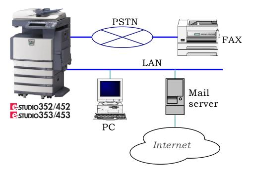
Figure 1-1 Typical operating environment of the TOE
