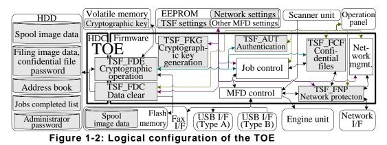
The TOE provides the following functions aiming to protect user data, including image data, etc. The purpose is to counter unauthorized attempts to obtain user data which are stored or remain in the non-volatile memory devices (such as the HDD) in the MFD. Another purpose is to counter attempts to wiretap user data when the MFD inputs and outputs the data over the network (LAN).
