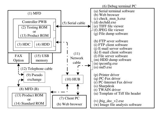
Figure 3-1: Configuration of the Developer Testing
