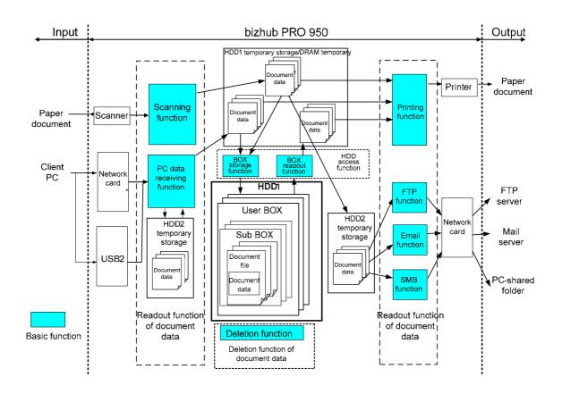
Figure 2.3 Processing Architecture of Basic Function
