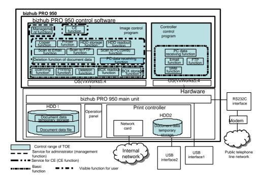
**Figure 2.2 TOE Structure**
