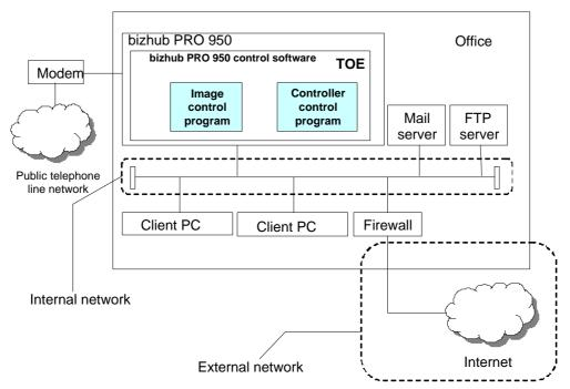
Figure 2.1 Operating Environment of bizhub PRO 950 Series
