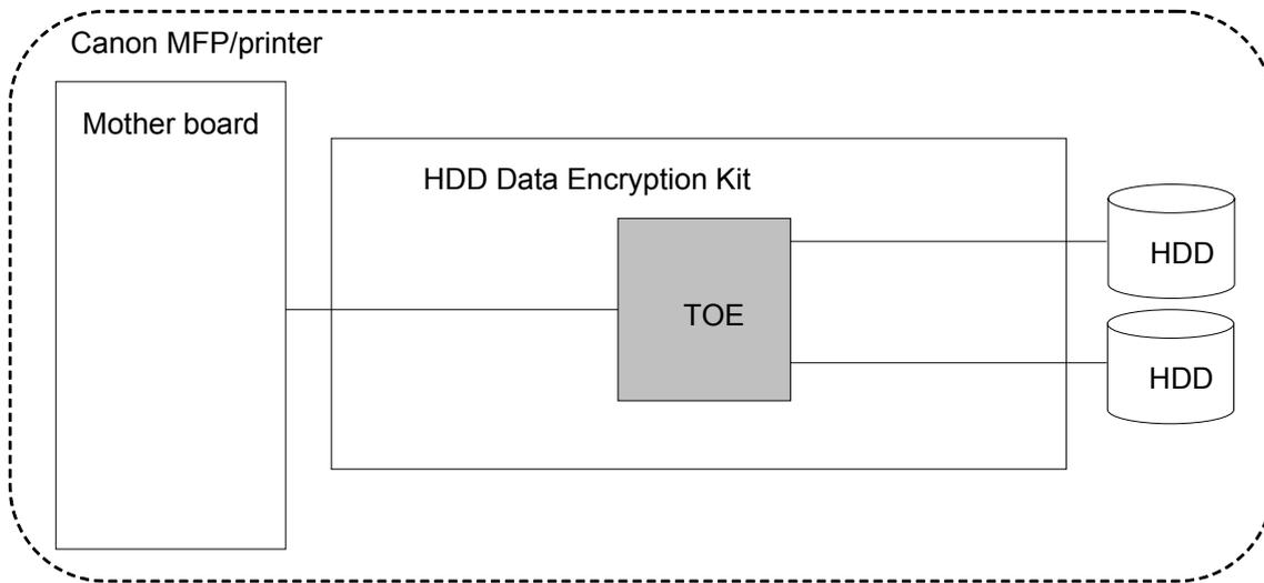
**Figure 2-1 : TOE usage environment**
