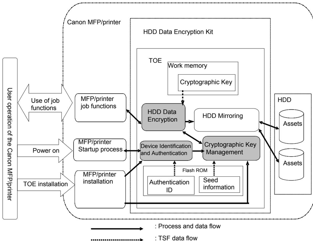
**Figure 2-3 : TOE logical configuration**
