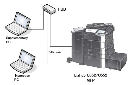
Figure 3-2 Configuration of Penetration Testing
