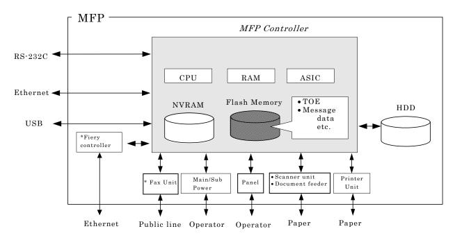
Figure 1-1 Hardware composition relevant to TOE
