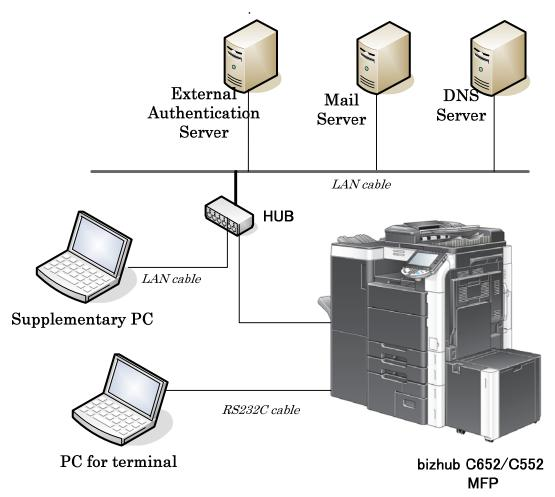
Figure 3-1 Configuration of Developer Testing
