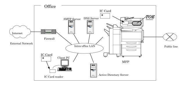
Figure 1 An example of MFP's use environments
