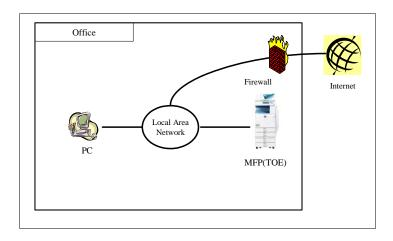
Figure 1: TOE Usage Environment
