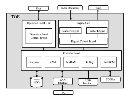
Figure 2: Hardware Configuration of TOE
