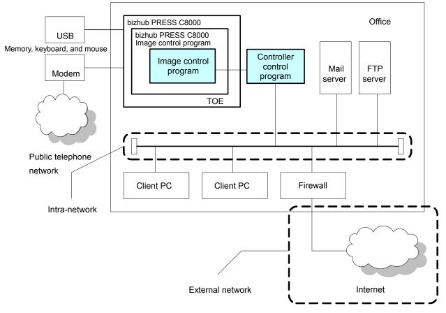
Figure 1 An example of the bizhub PRESS C8000 use environments
