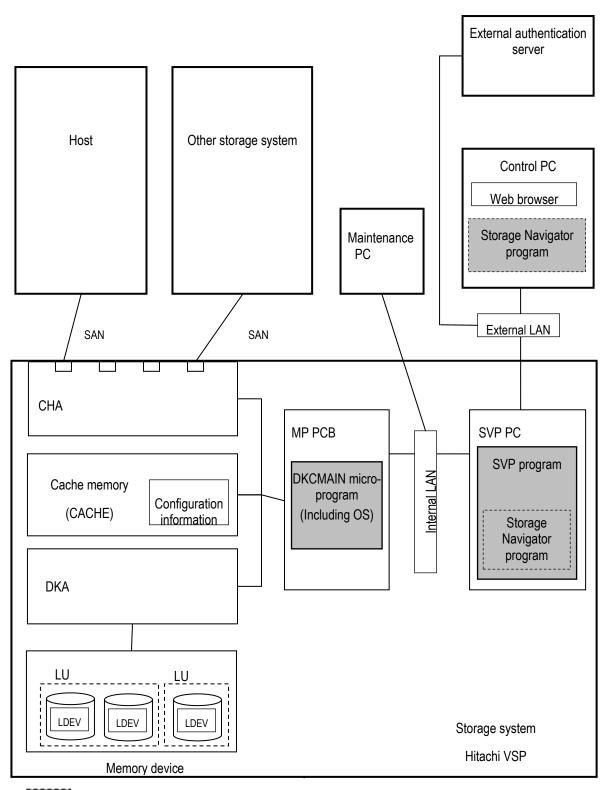
Storage Navigator program consists of Flex application and Java applet, and runs on SVP and control PC.
