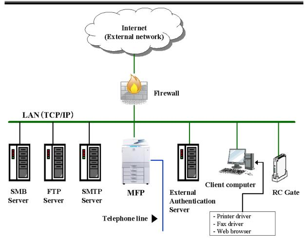
Figure 1 : Example of TOE Environment
