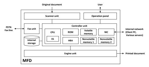
Figure 2: Physical configuration of the TOE
