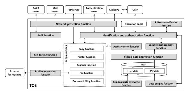
Figure 3: Logical configuration of the TOE
