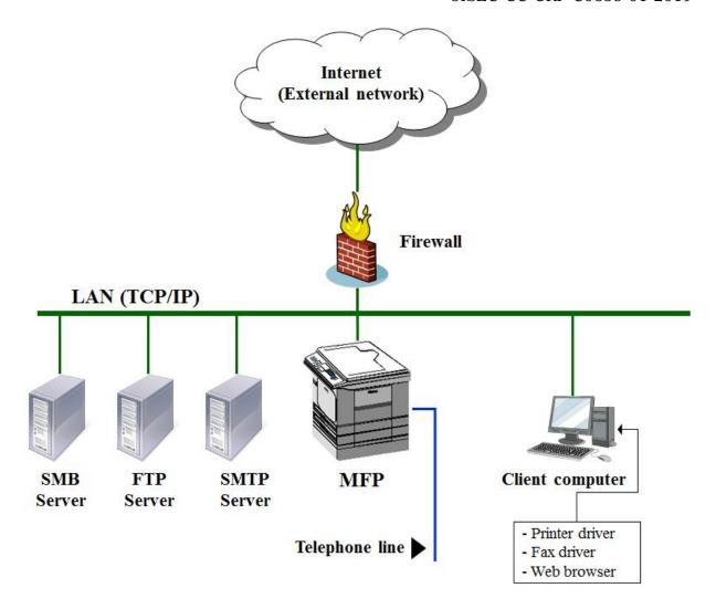
Figure 4-1 Operational Environment of the TOE
