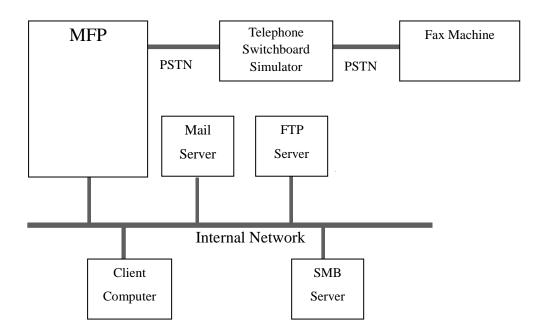
Figure 7-1 Configuration of the Developer Testing
