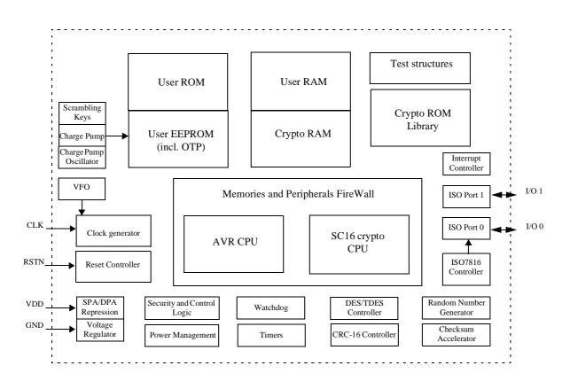
Fig. 2.1 -VEGA2 AT90SC19264RC Block Diagram
