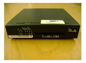
The TCRX2 contains the same monocard than the CRX (with a higher throughput) and the power supply is included into the box. Unless explicitly indicated, we will not distinguish the TCRX and TCRX2 in the present document (and we will simply indicate TCRX to refer to the two equipments).
