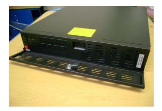
The TCRX is a monocard system including a network processor (Intel EGLXT973QCA3V) and a cryptographic processor (Altera EP1C20F324C8N).
