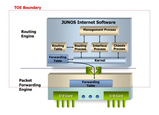
The interfaces to the TOE are twofold: the switching/routing interfaces and the management interfaces. The management interfaces include the TOE console interface through which the appliance can be managed locally and the in-band management interface via the network interfaces.
