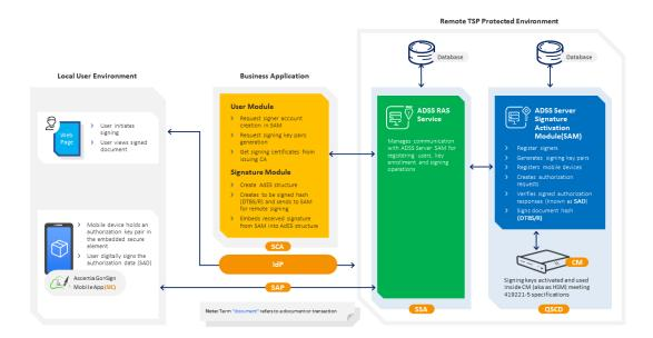
It is important to note that all API interactions with the ADSS Server SAM must be conducted through the ADSS RAS Service. This means from the perspective of the TOE, the ADSS RAS Service is considered as a Business Application. The TOE authenticates the ADSS RAS Service as a Business Application before allowing access to its services. Throughout this document the term Business Application applies to the ADSS RAS Service as well.
