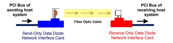
Figure 1 - High Level view of the Data Diode Interface
