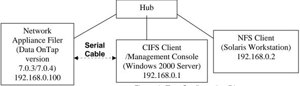
Figure 3: Test Configuration Diagram
