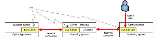
**Figure 2 TOE Architecture**
