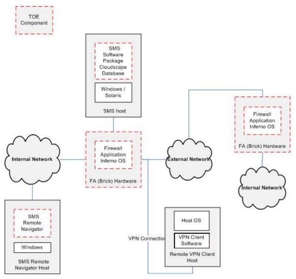
Figure 5: Physical TOE Boundary and Environment
