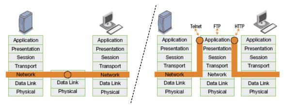
Figure 1-8- Traffic filtering (left) vs. Application-level Proxies
