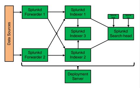
Figure 2 – TOE Deployment
