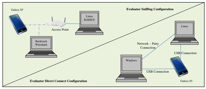
Figure 2 Evaluator Test Setup
