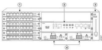
Figure 3 ASR 902 chassis design
